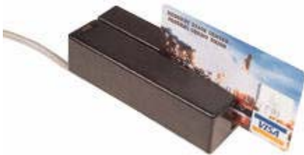
An Externally mounted Credit Card Slot Reader.
